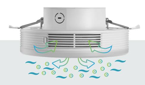
Airborne particles are charged by the ions released by the plasma generator, causing them to cluster, be drawn to the plasma and destroyed. This ionized air that contains positively and negatively charged molecules attract and kill airborne germs on contact.
