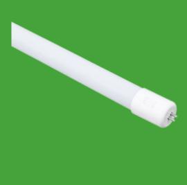
The ETi 22 watt 3300 lumen 4' integral LED T5 capped tubes offers exceptional versatility and performance for precision lighting applications that require the efficiency of a higher performance lamp. With the T5 connectors users can easily upgrade existing fixtures to a higher rated with minimal effort and maintenance. Dimmable with most brands.
