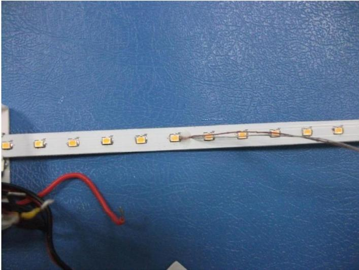
Thermocouple contact photograph(TMP<sub>Driver</sub>):
