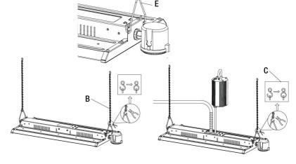
Connect the V Clips to each end of the fixture housing.
