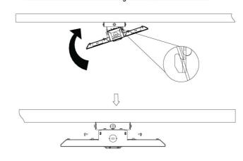
6b Connect the fixture housing to the mounting bracket and secure with 2 screws on each side.
