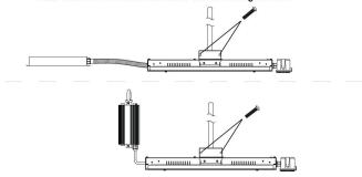
**6C** Connect the fixture housing to the mounting bracket and secure with 2 screws on each side.
