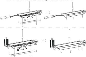
7c Make the electrical connections. See step 8a and 9a in the Suspension Mounting Installation section.
