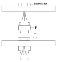
**4b** Feed wires from the electrical box through the mounting bracket. Use the electrical box screws to secure the mounting bracket to the electrical box.
