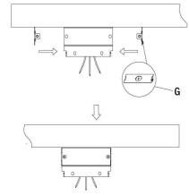
Attach the mounting bracket cover plates to the each side of the mounting bracket
