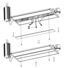
7b Make the electrical connections. See step 8a and 9a in the Suspension Mounting Installation section.
