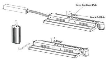
Remove the driver box cover plate from the fixture housing.
