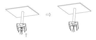
Feed the wires from the downrod through the mounting bracket and use a nut to secure the mounting bracket to the downrod.
