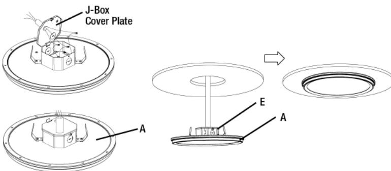
**8b** Feed wires through the knock out on the J-Box Cover.
