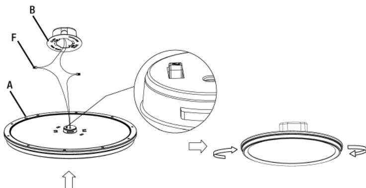
**8a** Secure the fixture to the mounting plate by inserting the fixture into the mounting plate and twisting the fixture until it is secure.
