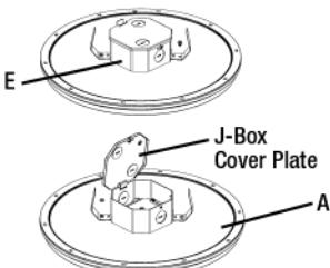
**6b** Use the 2 mounting plate screws to secure the J-Box with clips (not included) to the fixture housing.
