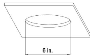
**5b** Find the desired mounting location and drill a 6 in. hole large enough to insert the fixture housing into the mounting location.
