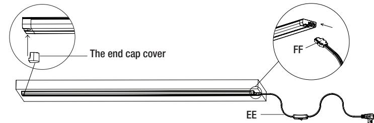
**3a** Connect the cord and plug assembly to the fixture and plug into the appropriate wall socket. Turn on the fixture using the toggle switch.
