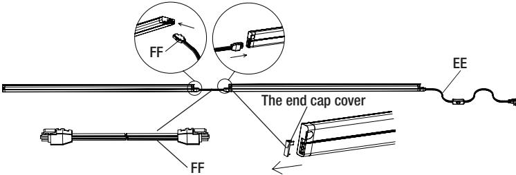
Remove the end cap cover and connect the fixture linking cables between the two fixtures per the diagram above.
