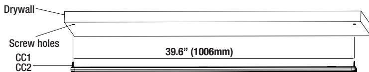
**2a** Drill pilot holes for direct screw or drywall anchors (as needed). On-center distance of the two mounting holes is (39.6" or 1006mm). Mount the fixture and re-install the screw hole access covers. (Installing contractor responsible for using the correct screws and/or anchors per the mounting surface.)
