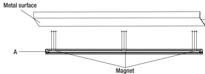
**1b** Fixture includes (3) high strength magnets suitable for installation to compatible metal surfaces for easy screwless installation.
