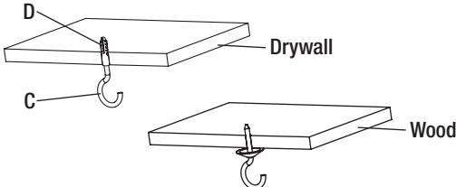
**3** If mounting to drywall: Drill two 1/4in. holes in the ceiling. Install the drywall anchors and the hook screws in each drilled mounting holes.
