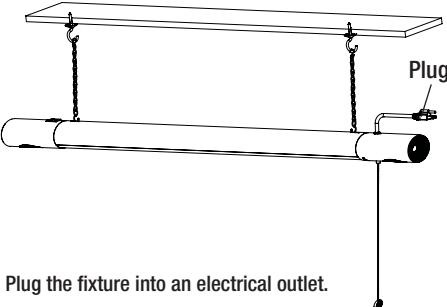
**7** Plug the fixture into an electrical outlet.
