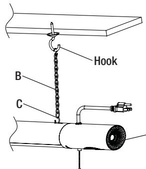
**4** Attach the S hooks that are at the bottom of the mounting chains to the fixture. Use pliers to close the S hooks and make sure the fixture is secure.
