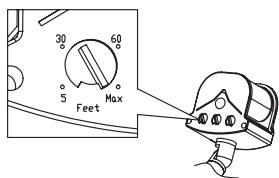
**13** Adjusting the sensitivity of the motion sensor:
