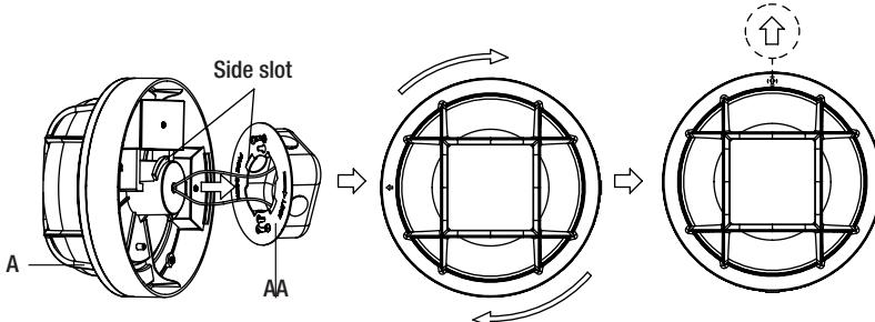
**2** Pass the hot and neutral (black and white) wires from the electrical outlet box through the middle hole of the mounting bracket (AA). Align the mounting bracket (AA) using the mounting screws (BB) and tighten securely to the electrical box.
