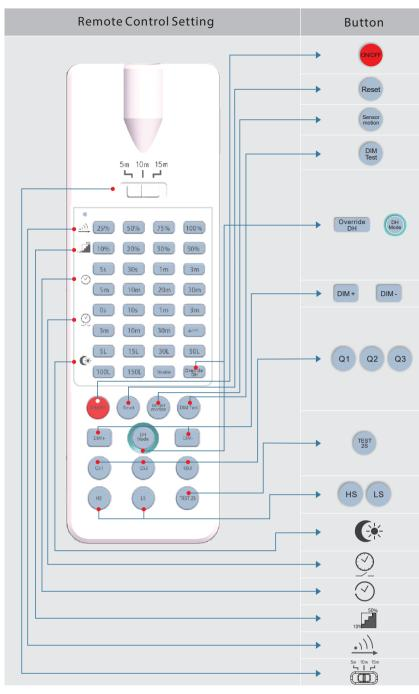
As the control angle of the Infrared Remote Control is fixed (15°), if sensors are installed too close to each other, settings of both sensors will be configured. Please refer to the below chart for the distance of the installation of the sensor:
