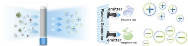
Low-energy Plasma Technology Electrons are released using a negative voltage of DC, and a material with superconducting properties is used as an electron release electrode to release a large amount of positive and negative ions.
