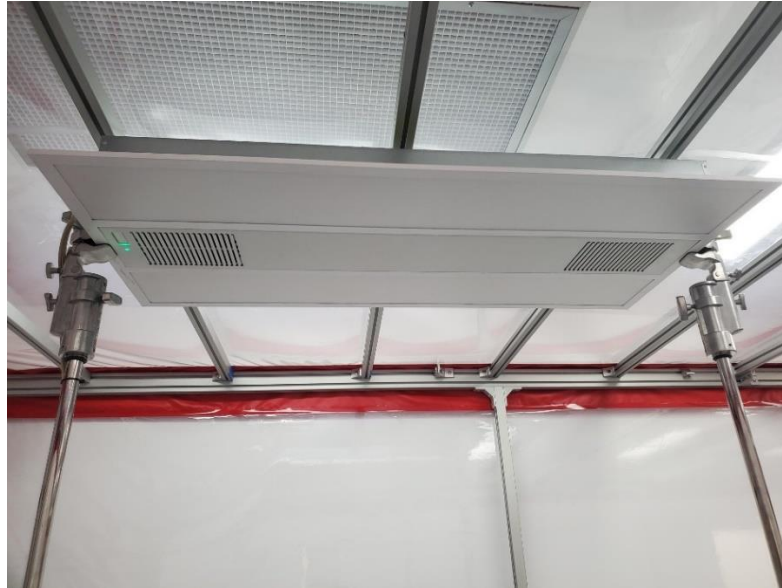
Figure 4. An image of the SilentAire Plasma 2x4 Troffer mounted in the center of the chamber for testing.
