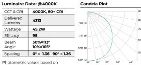
tests performed in compliance with LM-63 & LM-79
