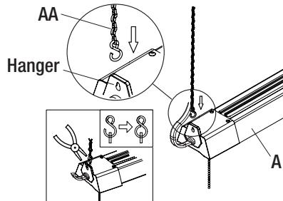
3. Hang the shop light (A) by placing one chain (AA) over each hook (CC) that has been installed on the ceiling.
