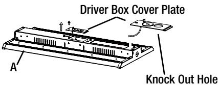
**3b** Remove the driver box cover plate from the fixture housing.
