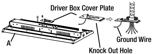
**3a** Remove the driver box cover plate and punch out the knock out hole.
