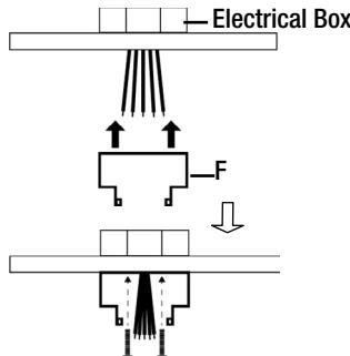
**4b** Feed wires from the electrical box through the mounting bracket. Use the electrical box screws to secure the mounting bracket to the electrical box.
