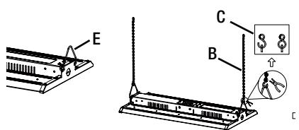
**5a** Connect the V Clips to each end of the fixture housing.
