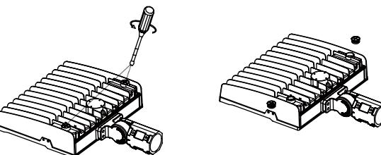
**2** After adjusting the required control function, tighten the metal plug and the plastic plug clockwise.
