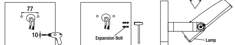
**ATTENTION:** When the photocell function is required, photocell should be installed on the back of lamp; When it's not required, shorting cap should be installed on the back of lamp.
