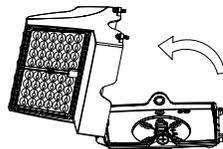
**3** Install the emergency led driver (EM) bracket onto the fixture.
