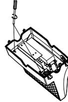
**4** Install the EM driver and battery on the bracket.
