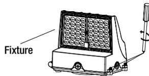
**2** Open the fixture and remove the heat sink.
