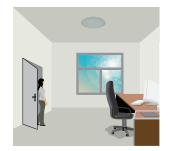
With sufficient natural light, the light does not turn on when presence is detected.
