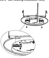
Replace lens and twist clockwise to lock.
