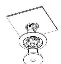
Replace lens and twist clockwise to lock.
