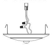
7a Screw E26 base adapter (not included) into socket in recessed housing, and simply slide the trim and metal friction clips into the housing.
