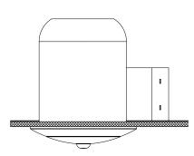
**9a** Caulk around the mounting surface edge with silicone sealant.
