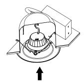
Tuck all the wires carefully into the can and push retrofit kit into can until flush with ceiling.
