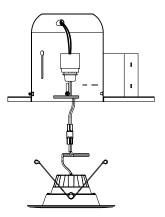
**7** Plug in the two plugs, the one from the socket adapter to the retrofit kit.
