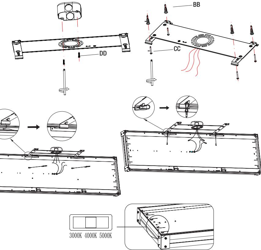
5. Level the top of the whole fixture (A) to the ceiling, then slide the fixture to the right, and confirm the fixture is secure.
