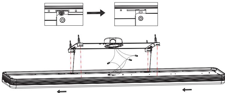
5. Level the top of the whole fixture (A) to the ceiling, then slide the fixture to the right, and confirm the fixture is secure.
