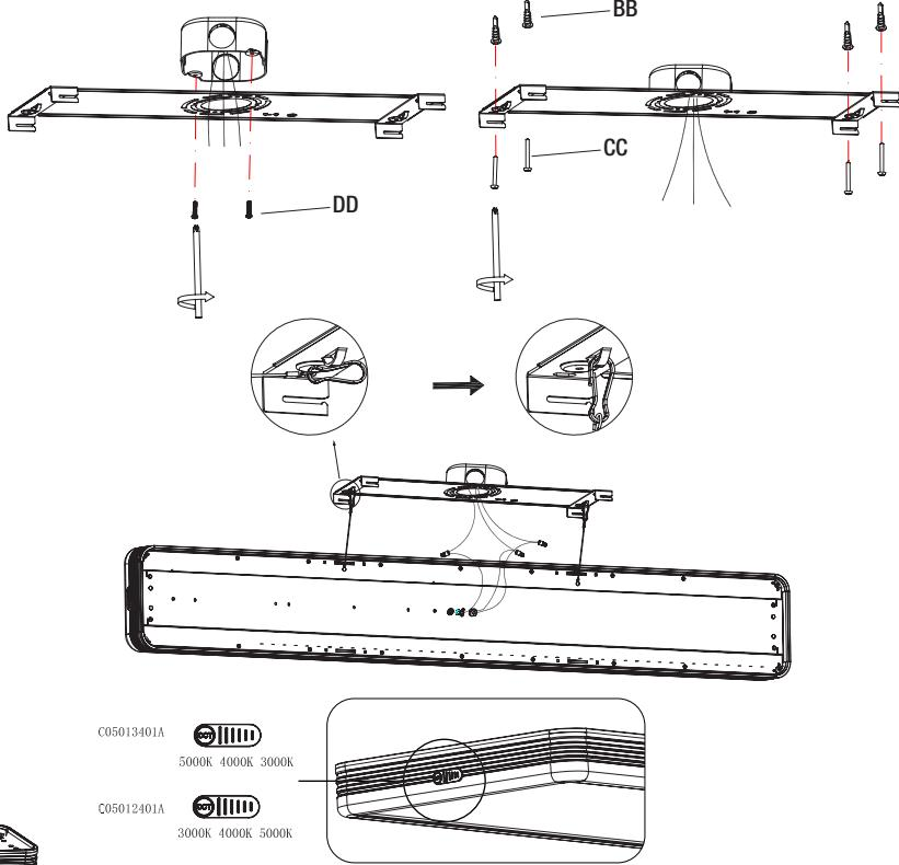
6. Turn on the power, and move the toggle switch to the desired color temperature.
