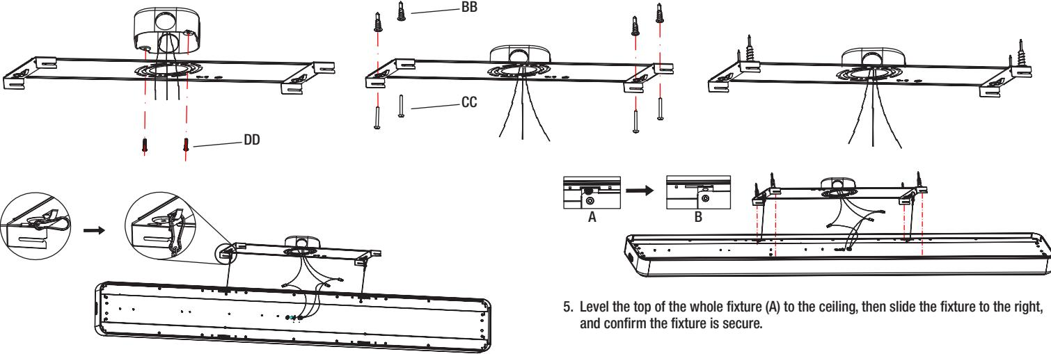
3. Hang the two holes on the left side of fixture (A) to the two hooks on the front end of mounting bracket (B) at the same time.
