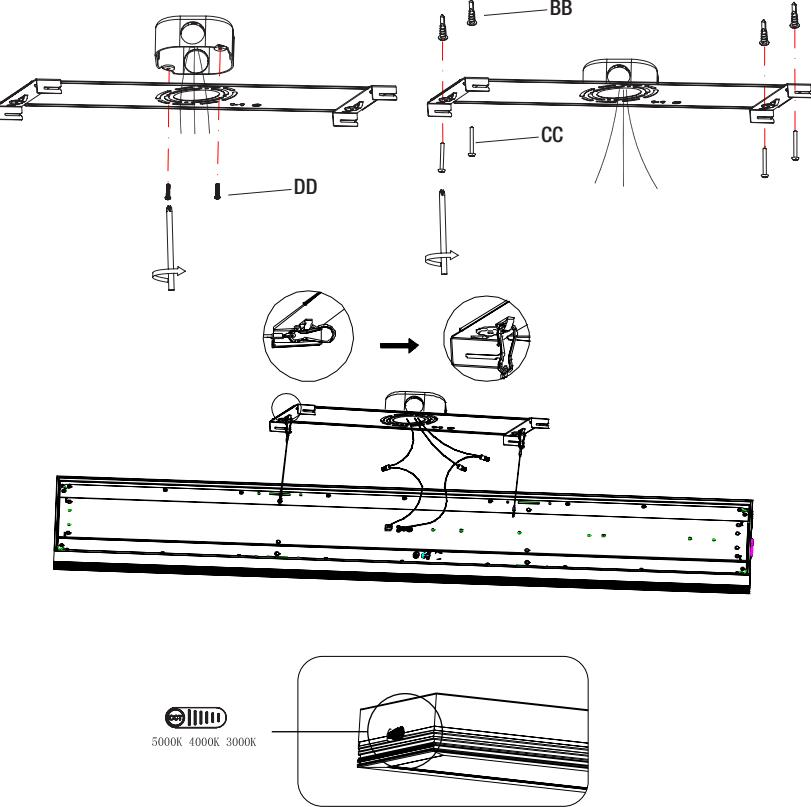
6. Turn on the power, and move the toggle switch to the desired color temperature.
