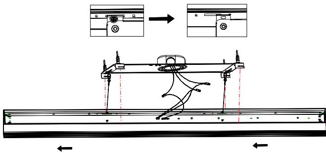
5. Level the top of the whole fixture (A) to the ceiling, then slide the fixture to the right, and confirm the fixture is secure.
