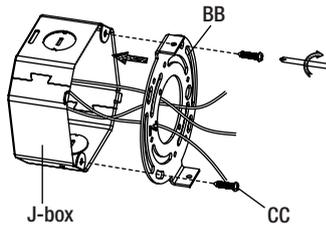
**2** Connect the hot and neutral (black and white) wires from the J-box to the same color wires from the fixture body (A). Wrap the ground wire from the electrical box around the ground screw on the mounting bracket (BB), then connect to the green wire from fixture body (A). Cover the wire connections using the wire connectors (AA). Cover the wire connectors (AA) with electrical tape for a more secure connection, then position the wires back inside the J-box.
