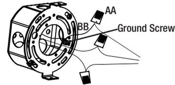
**3** Position the screw hole of the fixture body (A) face up, then place the fixture body (A) on the bracket (BB), ensuring it is close to the wall. Screw the fixture body (A) to the bracket (BB) using the mounting screw (DD).
